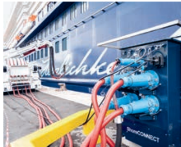
Wherever possible, our ships draw upon onshore electricity – an important contribution to reducing emissions.
